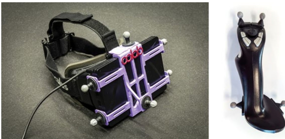
Figure 3. Wireless head-mounted display and joystick, both with markers attached for the motion-capture system.
